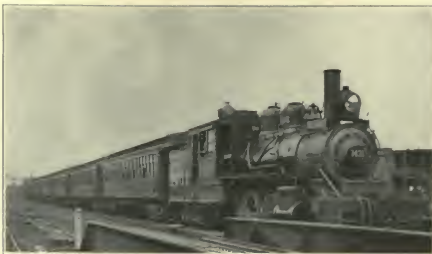
FIG. 369. SUBURBAN PASSENGER TRAINS. Flossmoor Suburban Train of the Illinois Central Railroad at the 67th Street Station. The train consists of a Forney type locomotive and six coaches.
